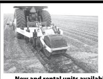
**Patriot Pivot** track closer fills in wheel ruts left by center pivot irrigation wheels.
